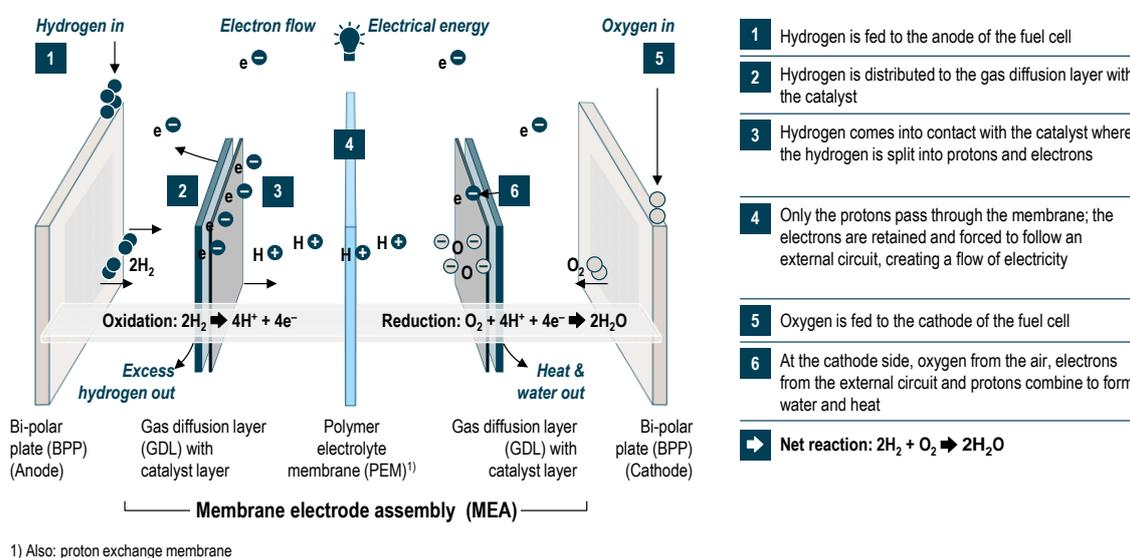
Figure 2: Schematic view of a polymer electrolyte membrane fuel cell (PEMFC)
