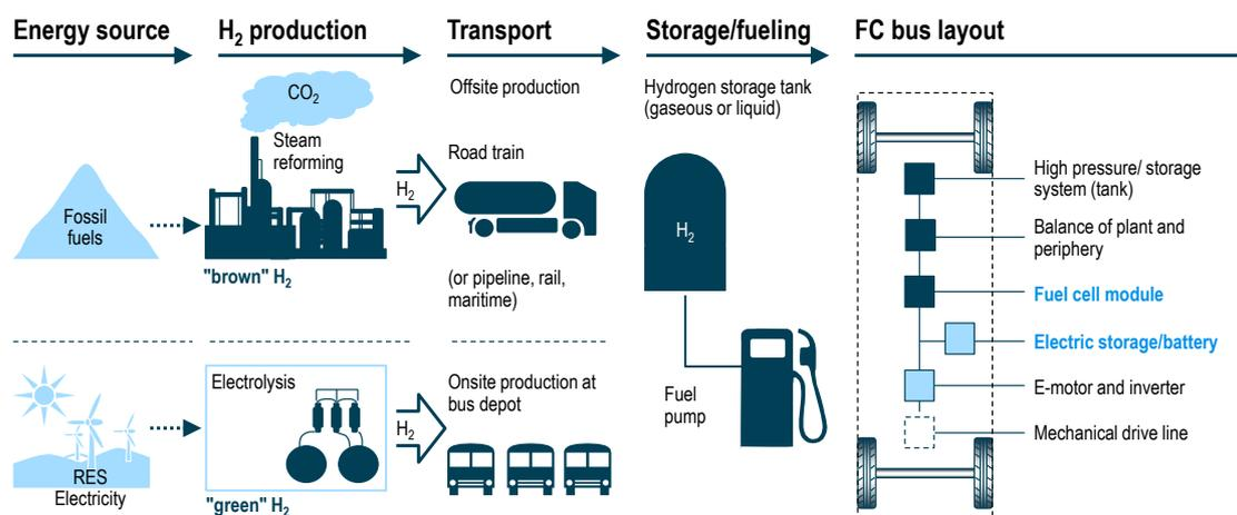
Figure 3: Hydrogen value chain and FC bus layout (simplified representation)
